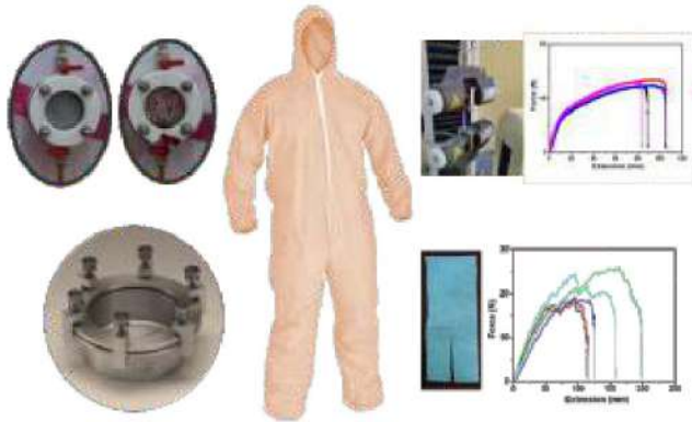
Fig. 1. Tests of Personal protective equipment for medical use. EN 29073-3 outlines the details of tensile testing. The PPE samples to be tested have to be prepared and conditioned before testing as per the international standards (ASTM D1776 and ISO 39). After conditioning, the specimens shall be tested using a calibrated UTM. Take note of the maximum breaking strength of the specimen in newtons (N), and the elongation corresponding to the ultimate breaking strength is recorded as the percentage of the nominal gauge length. For recording the tensile behaviour of wet specimens, the specimens have to be incubated in an aqueous solution of a non-ionic surfactant for a specific time period. After wetting, the specimens shall be analyzed immediately.
