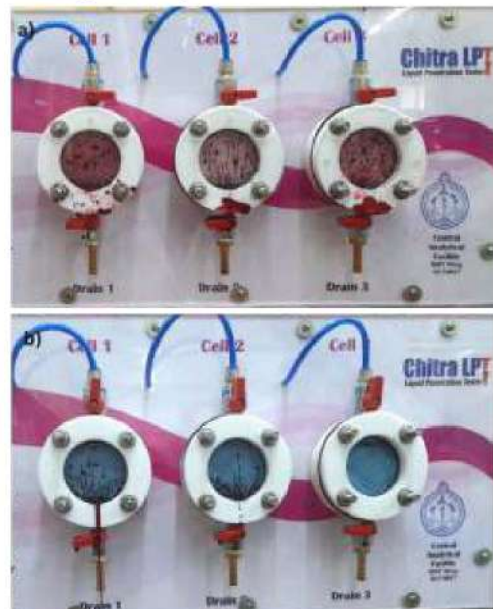
Fig. 2. Synthetic blood penetration test of PPE.
