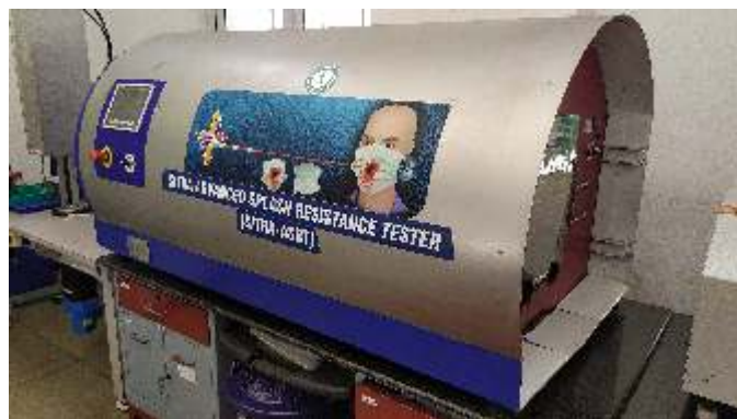
SITRA's in-house developed Advanced Splash Resistance Tester for Face masks
